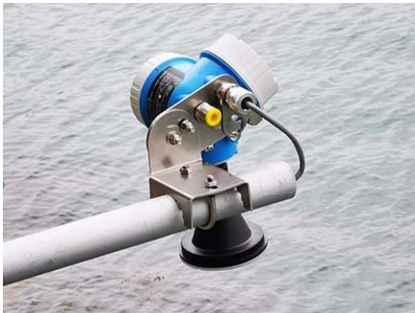
Radar water level sensor (Sontek, Xylem, USA) (left) and Dual Channel Echo-Sounder (Teledyne, USA) (right) used for hydrographic survey
