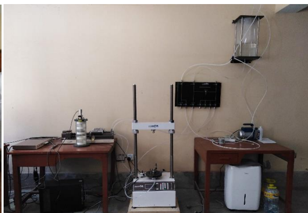
Visual inspection and scrutinized disturbed soil samples for simultaneous testing (left) Consolidation triaxial testing using Electro Mechanical Triaxial Testing machine (right)
