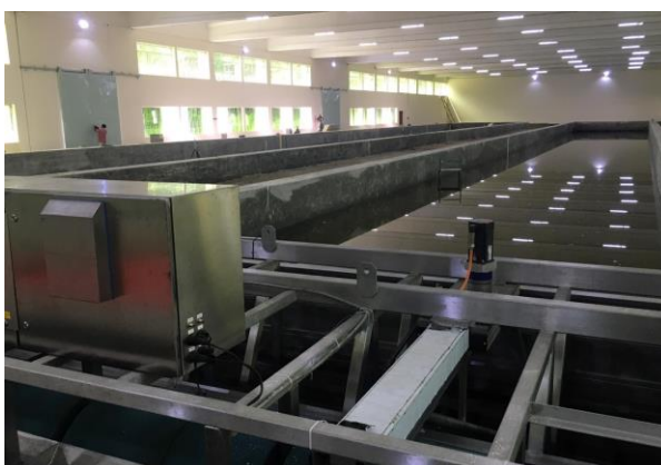
Recently commissioned 2D Wave Generator (HR Wallingford, UK) in the RRI Hydraulic Lab to facilitate coastal physical model study (supported by IDCB Project, Phase-II)
