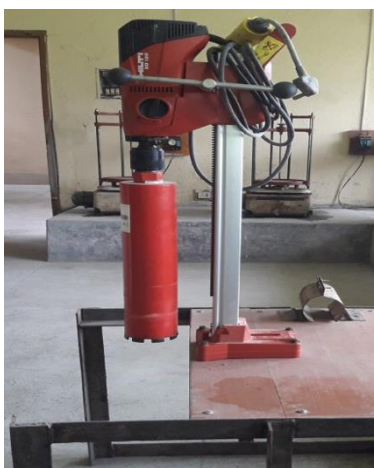
Recently purchased equipment (supported by IDCB Project, Phase-II) for Concrete and Material Testing Laboratory: Concrete crushing machine (Controls, Italy) (left) and Core cutter machine (Hilti, Switzerland) (right) used for cutting concrete block and extract core.
