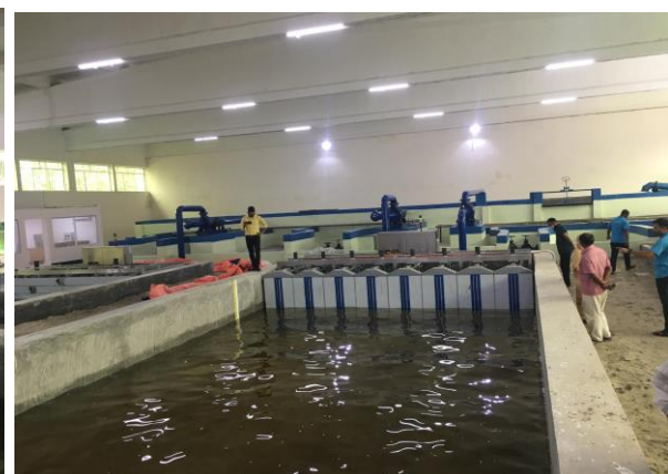
2D Wave Generator (HR Wallingford, UK) (left) and Tide Generator with 3D Wave Maker (HR Wallingford, UK) (right) used for coastal physical model study
