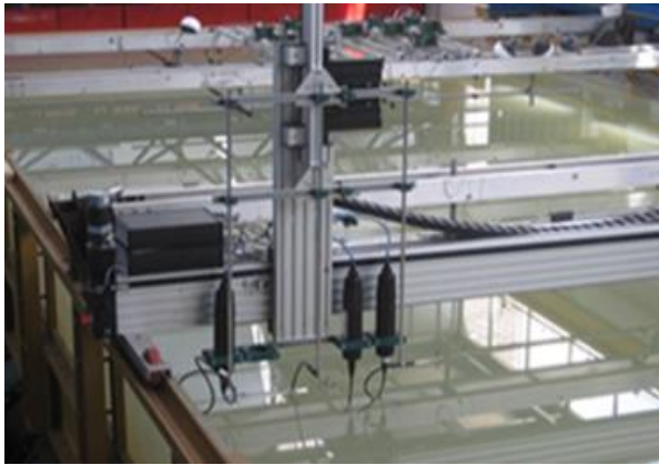
3D Bed Profiler (HR Wallingford, UK) (left) used for physical model study and ADCP (Sontek, Xylem, USA) (right) used for hydrographic survey
