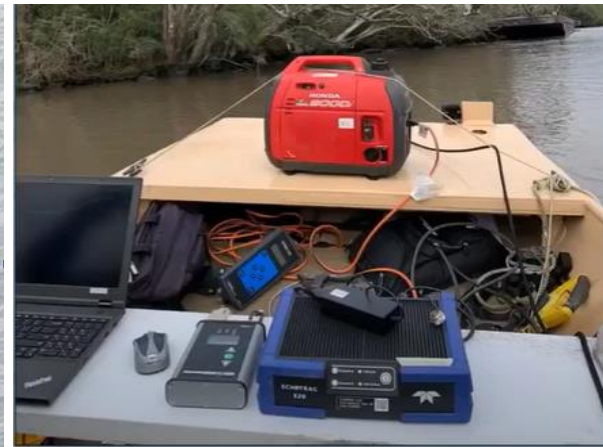
Radar water level sensor (Sontek, Xylem, USA) (left) and Dual Channel Echo-Sounder (Teledyne, USA) (right) used for hydrographic survey
