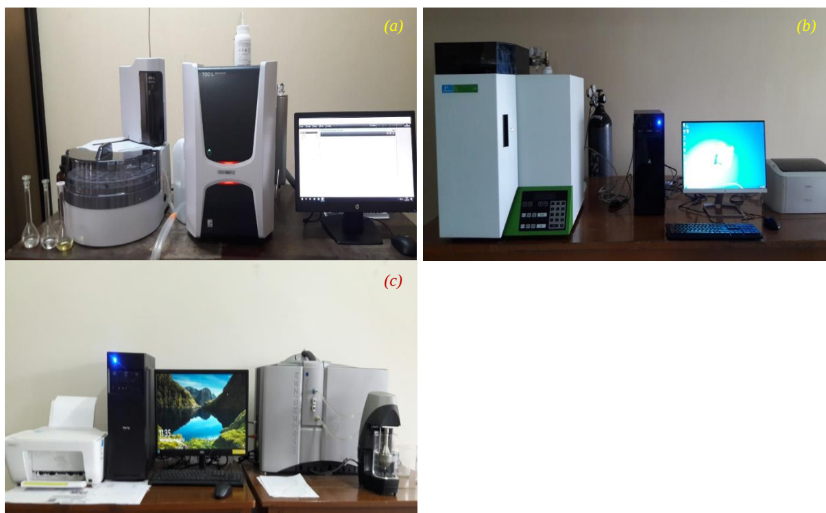
Recently procured equipment (supported by IDCB Project, Phase-II) for Chemical Laboratory: (a) TOC Analyzer, (Shimadzu, Japan) (b) CHNS Analyzer with air purifier, (Perkin Elmer, UK) (c) Particle Size Analyzer (Malvern Panalytical, UK).
