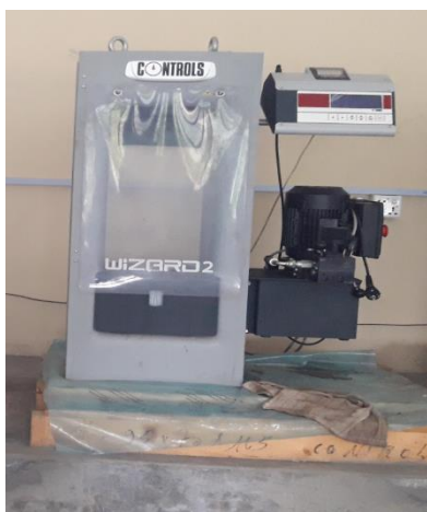
Recently purchased equipment (supported by IDCB Project, Phase-II) for Concrete and Material Testing Laboratory: Concrete crushing machine (Controls, Italy) (left) and Core cutter machine (Hilti, Switzerland) (right) used for cutting concrete block and extract core.
