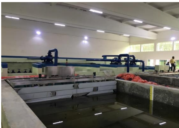
2D Wave Generator (HR Wallingford, UK) (left) and Tide Generator with 3D Wave Maker (HR Wallingford, UK) (right) used for coastal physical model study
