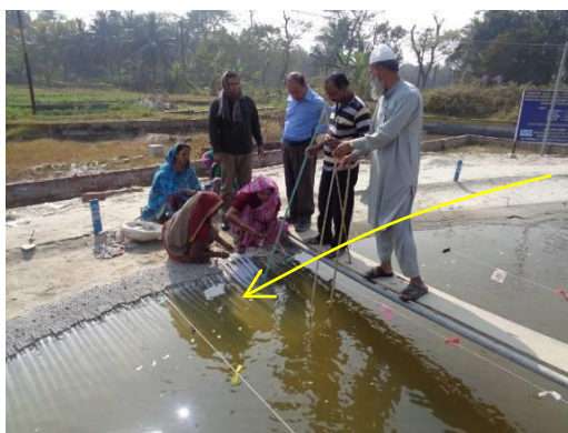
Figure 1: Placement of CC blocks during low flow in the model
