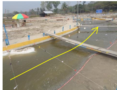
Figure 2: Model is under running condition with oblique flow
