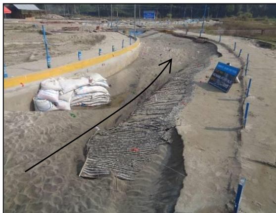
Figure 3: Scour pattern in the vicinity of CBM and oblique char
