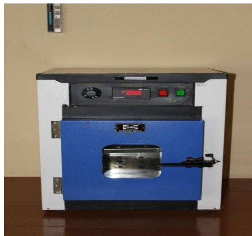
Incubator used to maintain required temperature of reagents and samples.
