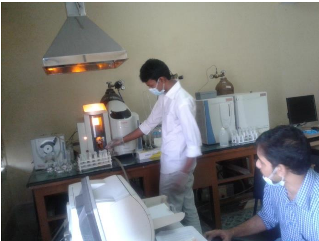
Heavy metal detection in water samples using Atomic Absorption Spectrometer at Chemical Lab
