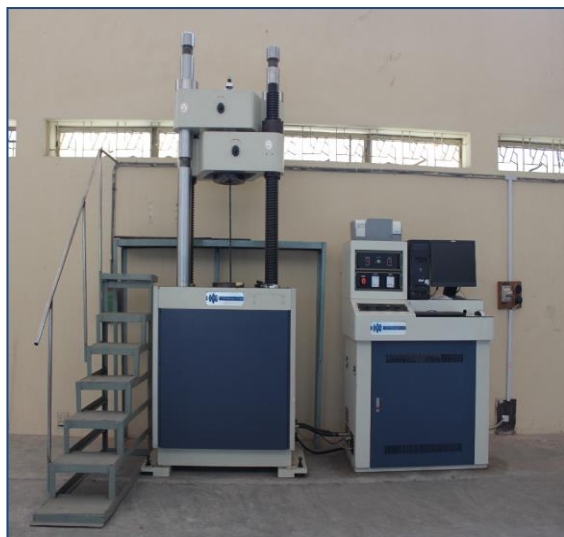
Universal testing machine for testing of MS rod, flat bar, concrete cylinder, block etc.
