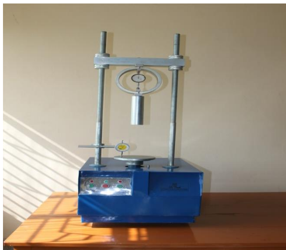
CBR test equipment to determine bearing capacity of soil
