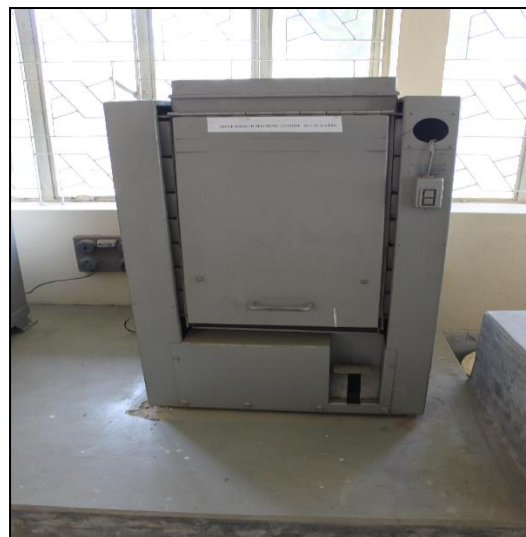
Sieve Shaker for gradation analysis of coarse aggregates
