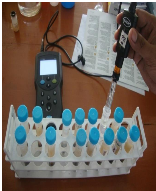
pH measurement of sediment samples using HACH 30QD multiparameter meter in chemical
