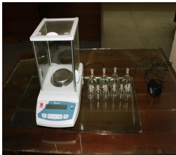
Equipment for determining specific gravity of soil
