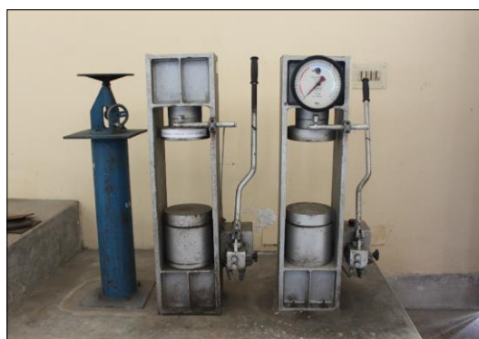
Compressive strength testing machine used for testing of concrete cylinder, block etc.
