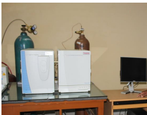
Gas Chromatography-Mass Spectroscopy for detecting volatile organic compound in soil and water.
