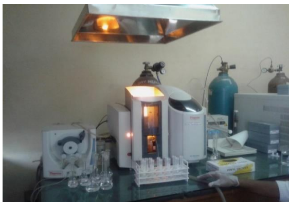
Atomic Absorption Spectrometer for detecting heavy metals such as Zn, Al, Pb, B, Cd, Cr, Mg, Fe, As, Hg etc in soil samples.
