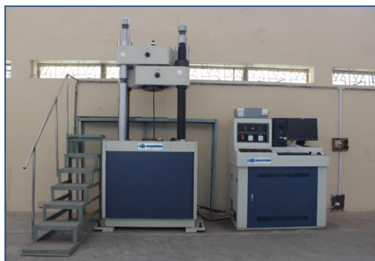
Universal testing machine used for testing of MSrod, flat bar, concrete cylinder, block etc.
