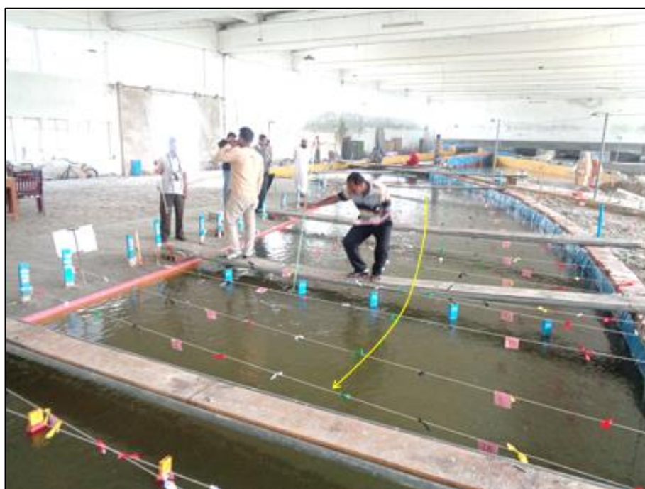
Figure: A view of physical model study of Bangabandhu Railway Bridge Project during running condition.
