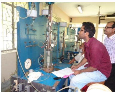
Laboratory shear strength investigation by triaxial shear test apparatus
